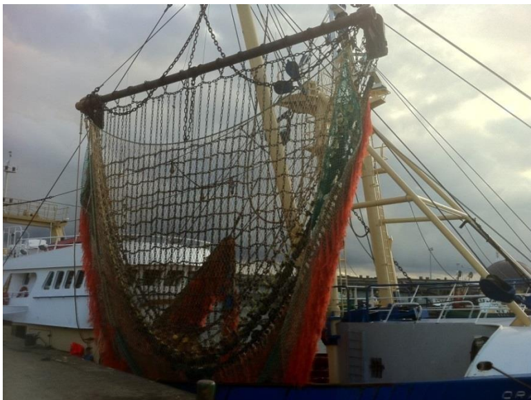
Plate A13.2.7 A traditional beam trawl net with tickler chains and chain mat (BMM, 2012)
