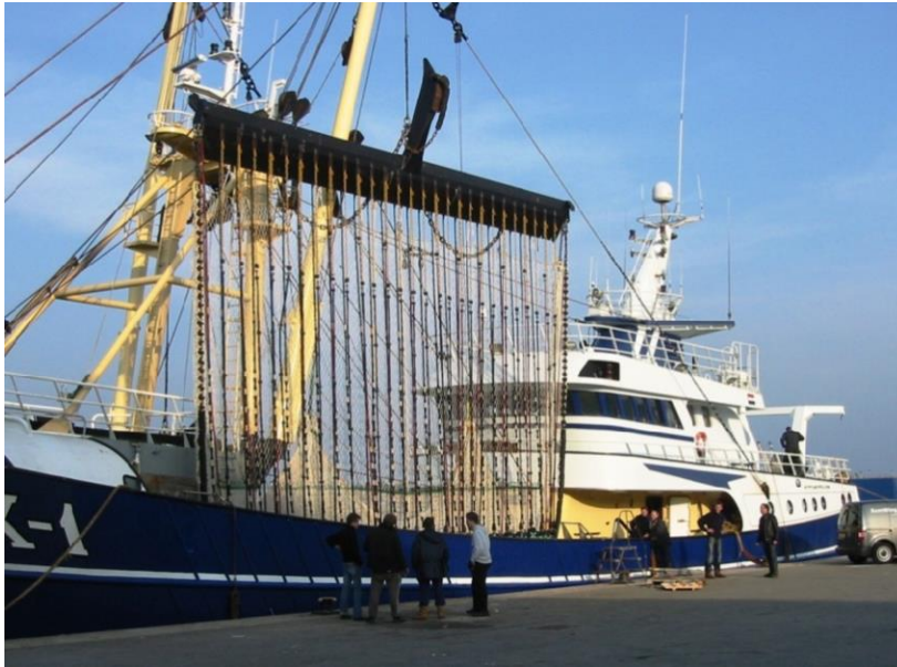
Plate A13.2.8 A Dutch fishing vessel with a pulse wing trawl (Eayrs & Suuronen, 2013)
